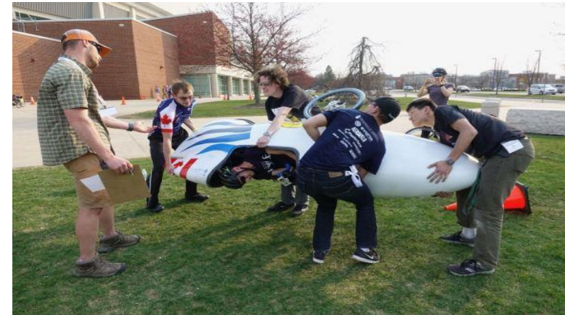
Figure 6: Roll Cage Rollover Safety Test
